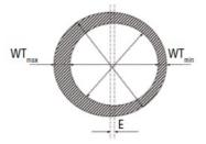
E is half of the difference between biggest and smallest wall thickness (WT) values in one cross section.
